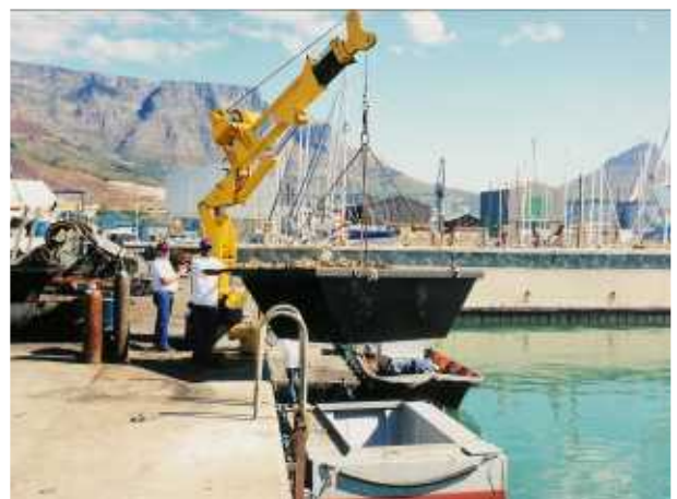
Transfer Skips can be loaded by crane or truck
