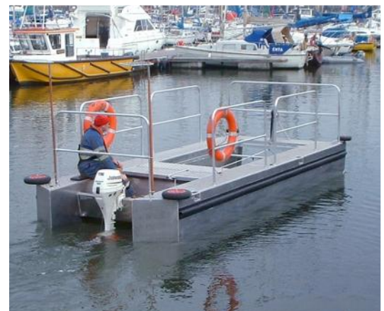
6m Buddy with tiller-controlled 15hp engine
