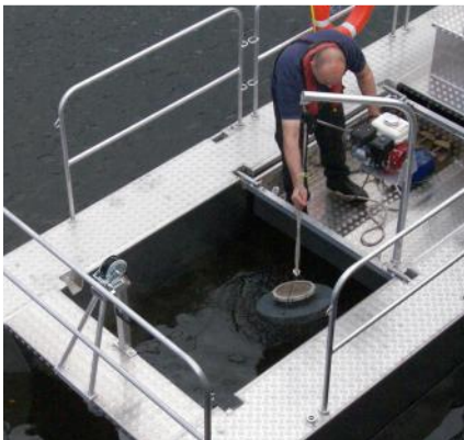
Pot Puller / Davit With manual or powered winch.
