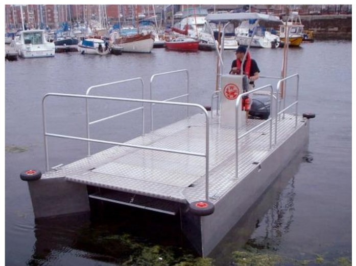
Deck plates provide a 13m 2 working platform
